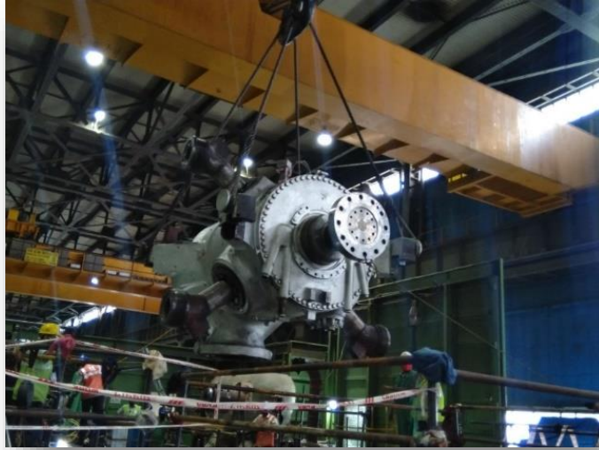
Refurbished HP turbine
