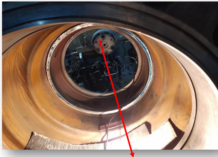
ABUTMENT FACE BLUE CONTACT AREA BEFORE LAPPING
